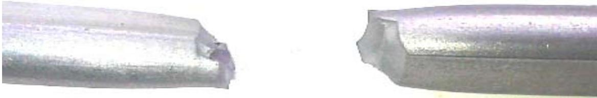
(b) Fractured experimentally RBS specimen.
