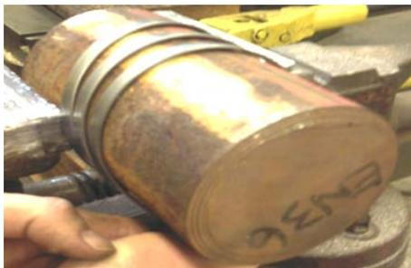
*Figure 2 :* Experimental simulation of reverse bending of tensile armour bar
