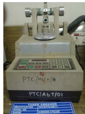
Fig. 2 : Experimental setup for Wear Resistance test.
