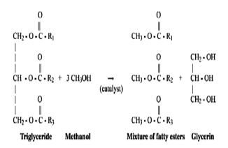
Figure 1: Transesterification of triglycerides with methanol to FAME
