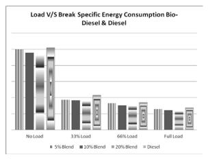
Fig 5: BSEC Vs Engine Load
