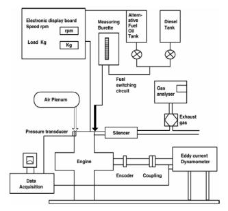
Fig. 2: Experimental Setup
