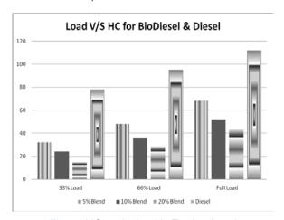
Fig. 8: HC emission Vs Engine Load
