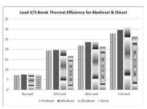
Fig.3: BTE Vs Engine Laod
