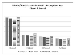
Fig. 4: BSFC Vs Engine Load
