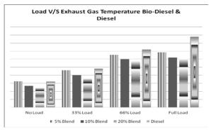
Fig 6: EGT Vs Engine Load
