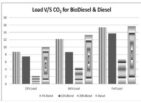
Fig. 9: CO<sub>2</sub> emission Vs Engine Load
