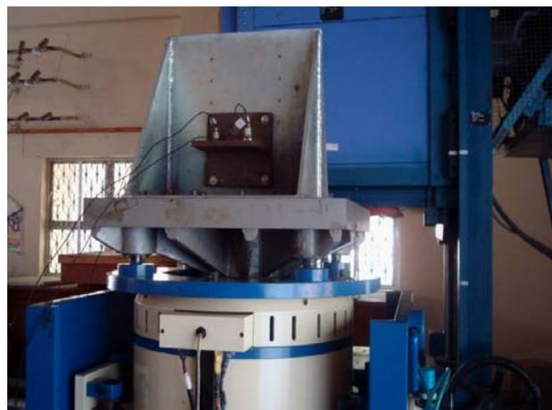
Fig.1 : Test Structure fitted to the Multi Axis Electro Dynamic Vibration Shaker
