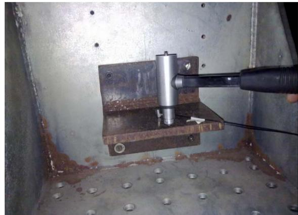
Fig. 3 : Experimental setup for Impact Hammer test
