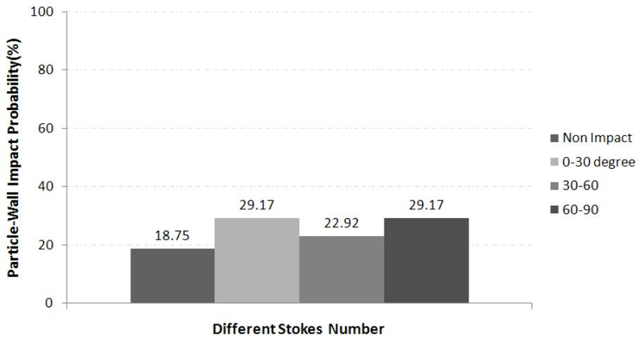
Fig. 8 : The particle impact probability at different area of bend wall for different Stokes number
