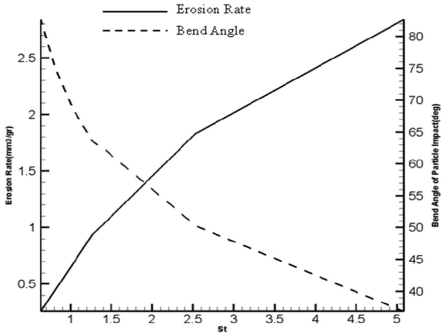
Fig11 : The particle impact angle and the erosion rate at the bend for different Stokes number
