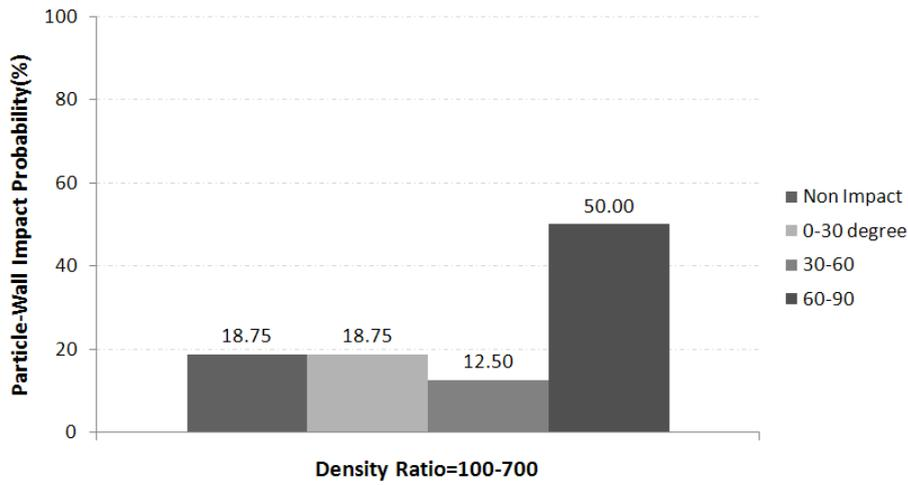
Fig. 7 : The particle impact probability at different area of bend wall by changing the density ratios
