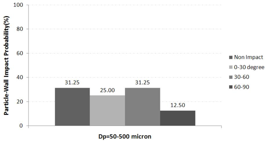
Fig. 6 : The particle impact probability at different area of bend wall by changing the particle diameter
