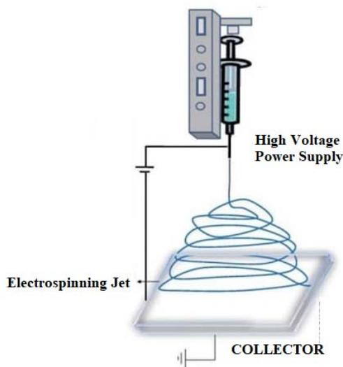
Fig. 9: Scheme of the electrospinning process
