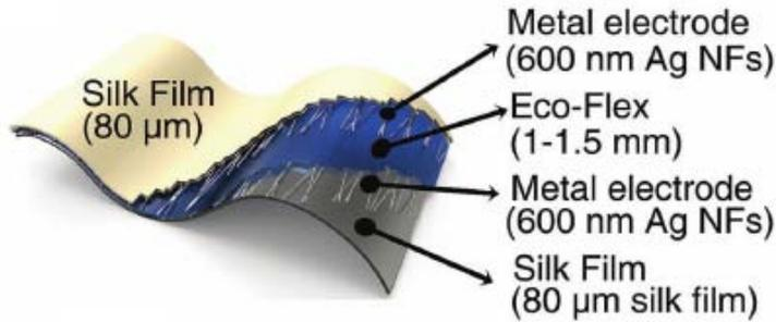
Fig. 15: Structure of the pressure-strain sensor from C. Hou et al. Small 2019
