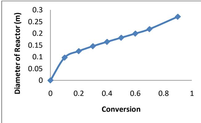
Figure 2: Plot of Diameter of Reactor versus Conversion
