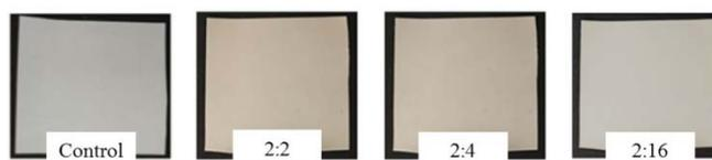
Figure 2: UH050 control and modified membranes with concentrations of DA/PVP of 2:2; 2:4; 2:16 mg mL<sup>-1</sup> and deposition time of 2h.
