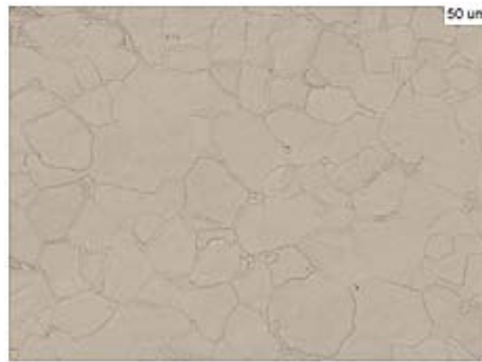
Figure 13: The microstructure of the middle sector (ferrite)
