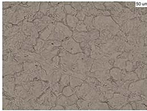
Figure 12: The microstructure of the lower sector (ferrite+perlite)
