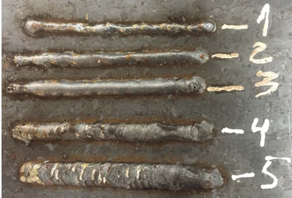
Figure 2: Deposited beads using different process parameters
