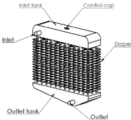
Fig. 1: Parts of a radiator
