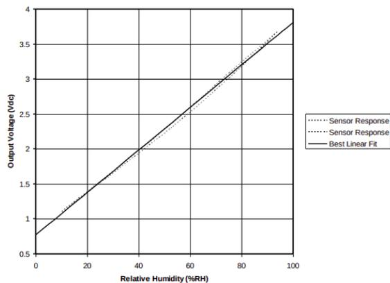
Figure 4: Relative humidity sensor response curve (HIH4000)
