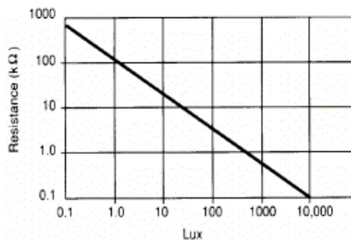
Figure 2: Brightness vs. resistance graph
