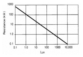
Figure 2: Brightness vs. resistance graph
