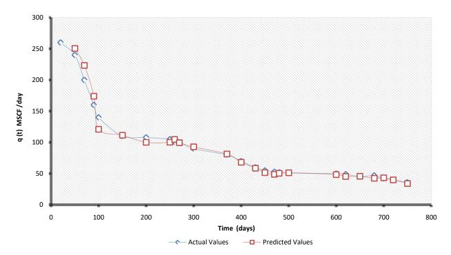
Figure 9: Graphical representation of actual flow rate vs. forecasted flow rate for shale gas production using the ARIMA model
