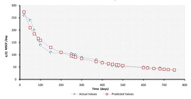
Figure 4: Graphical representation of actual flow rate vs. forecasted flow rate for shale gas production using the PLE model
