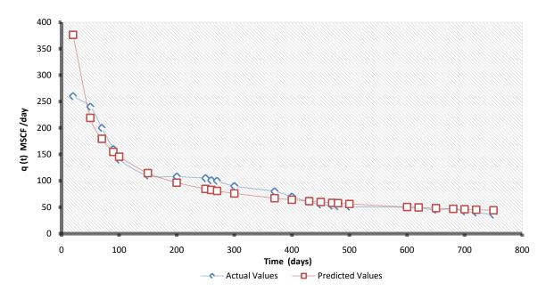
Figure 3: Graphical representation of actual flow rate vs. forecasted flow rate for shale gas production using Duong's model
