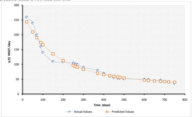
Figure 8: Graphical representation of actual flow rate vs. forecasted flow rate for shale gas production using the Duong-PLE hybrid model
