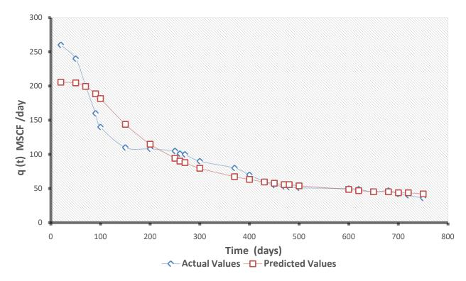
Figure 2: Graphical representation of actual flow rate vs. forecasted flow rate for shale gas production using the Arps model
