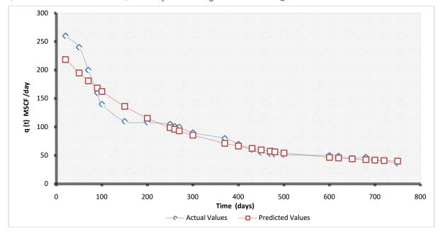
Figure 7: Graphical representation of actual flow rate vs. forecasted flow rate for shale gas production using the Arps-PLE hybrid model
