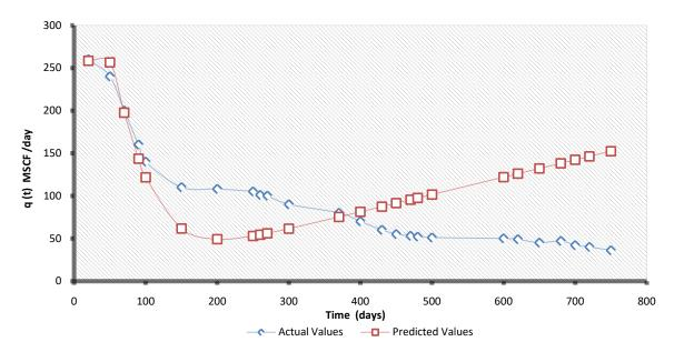
Figure 6: Graphical representation of actual flow rate vs. forecasted flow rate for shale gas production using the Arps-Duong hybrid model
