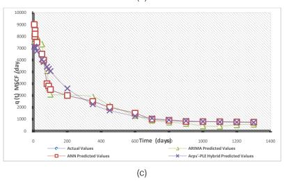
Figure 12: Estimated production data to determine accuracy of the different hybrid models (a), (b) and (c) ARIMA vs. ANN vs. Arps-PLE hybrid model [32;42;43]
