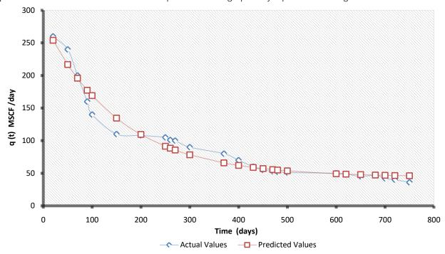
Figure 5: Graphical representation of actual flow rate vs. forecasted flow rate for shale gas production using the Arps-Duong-PLE hybrid model
