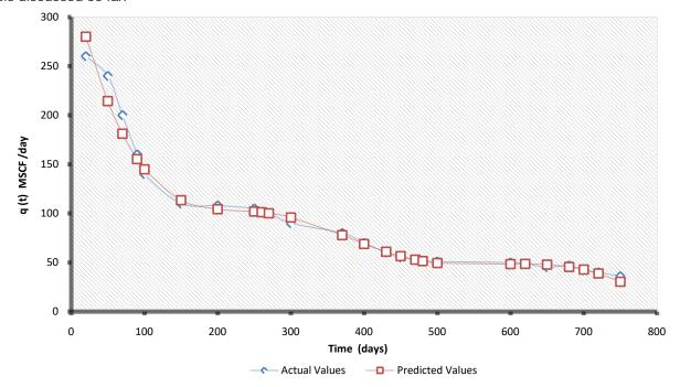
Figure 10: Graphical representation of actual flow rate vs. forecasted flow rate for shale gas production using the ANN model
