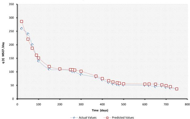
Figure 11: Graphical representation of actual flow rate vs. forecasted flow rate for shale gas production using the hybrid model
