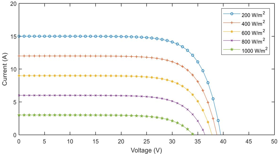
Fig. 10: Current-voltage characteristic for various radiation values  $I = f(V)$ ;  $T = 25C$
