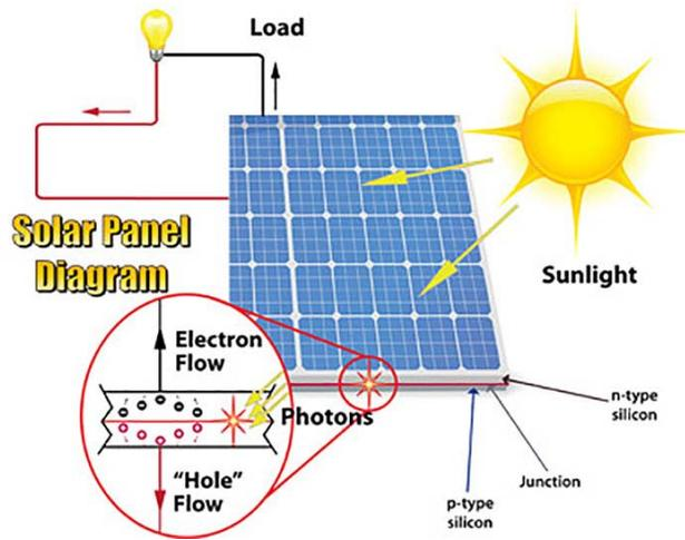
Fig. 1: Photovoltaic panel
