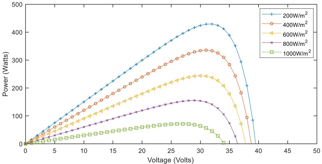
Fig. 11: Power-voltage characteristic for various radiation values  $P = f(V)$ ;  $T = 25\text{C}$
