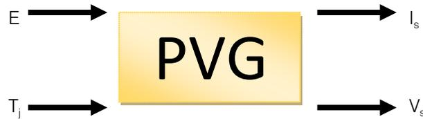
Fig. 3: Photovoltaic generator block diagram
