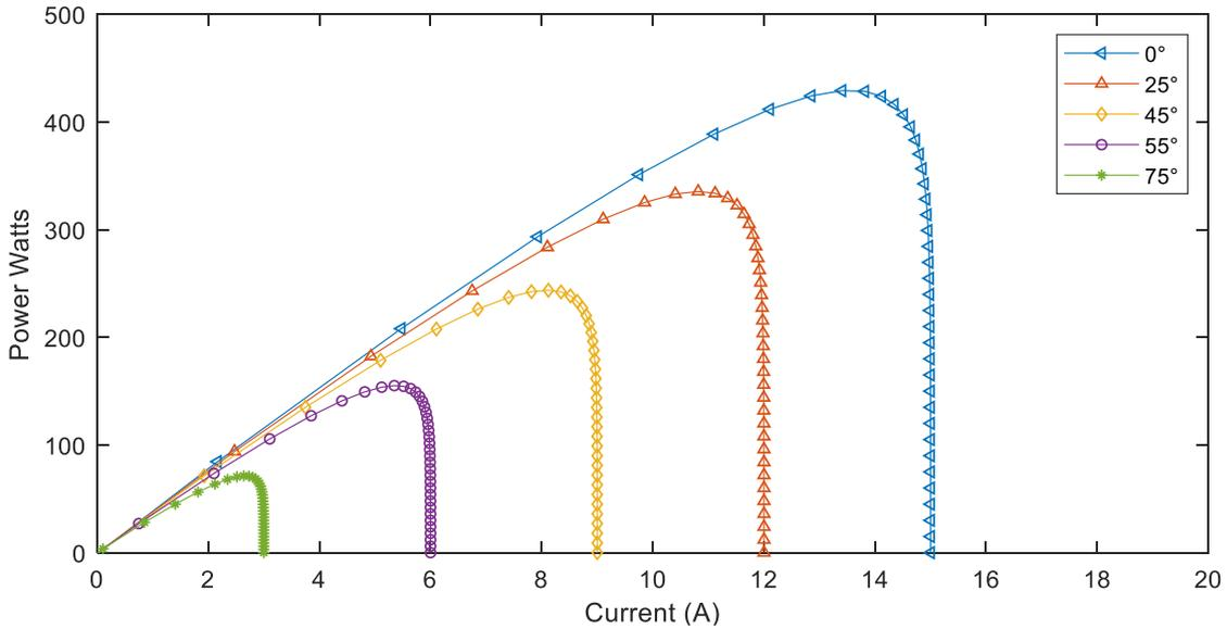
Fig. 9: Characteristic power-current for various values of the temperature  $P = f(I)$ ;  $E = 1000W / m^2$
