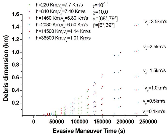
Figure 10: - Risk Curve - Debris dimension vs. Evasive Maneuver time.
