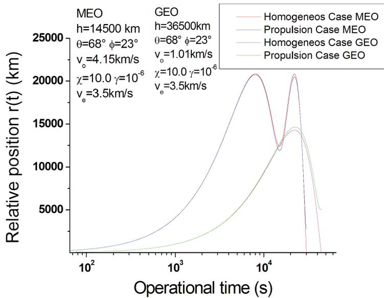
Figure 6: Relative position of the two objects as a function of time for different operational regions - MEO and GEO.
