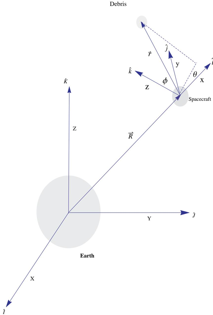
Figure 1: Reference frame for a vehicle around Earth and for a space debris. The frame with capital letters is positioned in the Earth center.
