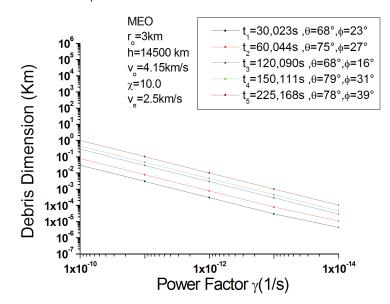
*Figure 7:* Behavior of the parameter vs. debris size vs. operation time, MEO.
