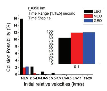
*Figure 4:* Collision Possibility in orbital regions vs. Initial relative velocities: 0.0 - 20.0 km/s,  $r_0$  = 350 km.
