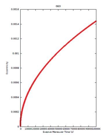
*Figure 12A:* Variation in the satellite eccentricity by the time. The satellite is in GEO, the gas exhaust velocity is 2.5 km/s, the mass factor of 10, the power factor of the engine is 10–10 1/s.
