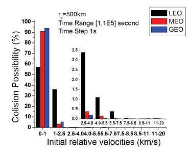
*Figure 5:* Collision Possibility in orbital regions vs. Initial relative velocities: 0.0 - 20.0 km/s,  $r_0 = 500$  km.
