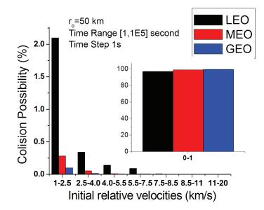
*Figure 3:* Collision Possibility in orbital regions vs. Initial relative velocities: 0.0 - 20.0 km/s,  $r_0 = 50$  km.
