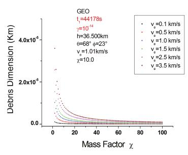
*Figure 9:* Debris Dimension vs. mass parameter,  $\chi$ ,  $\gamma = 10-14$  1/s, in GEO.
