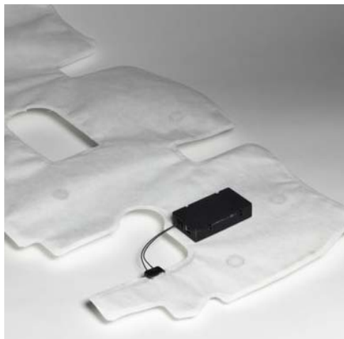
Fig. 4: Capacitive Sensor attached on felt
