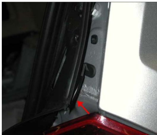
Fig. 7: Sensor Profile connected to wire-harness [2]
