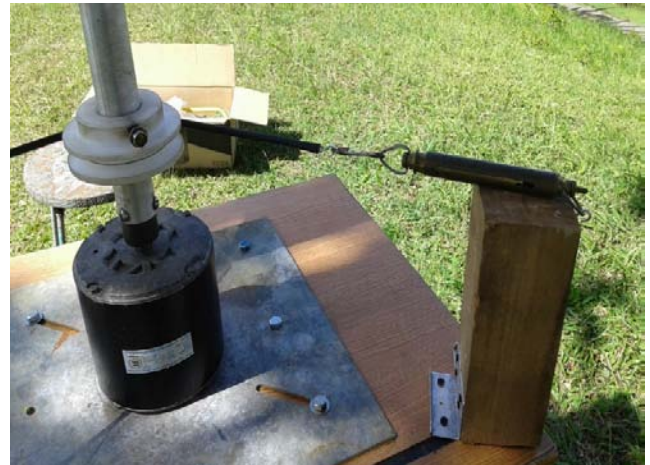
Figure 11: Showing the dynamometer built
