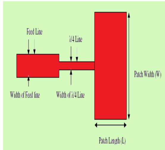
Fig. 5: Antenna Design with Feed-line, Patch & Transformer
