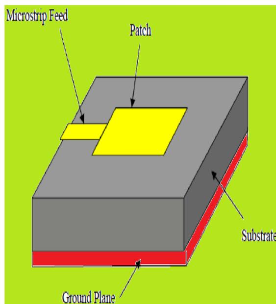
Fig. 1: Microstrip Patch Antenna
