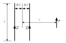
*Fig. 1:* Common mode noise equivalent model
