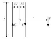
Fig. 2: Differential mode noise model
