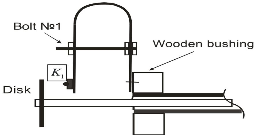
Fig. 19: Schematic of blanking sensor.
