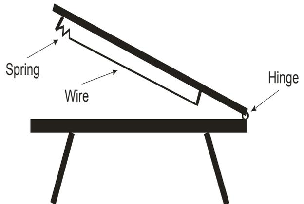
to the working table to the hinge is fastened the board, on which are located two metallic pintles. The Nichrome wire with a thickness of 0.5 mm. is extended between the ends of these pintles. So that with the heating the wire would not sag, spring is used. To the wire through the step-down transformer brings the stress, which is selected in such a way that the heated wire would rapidly melt foam plastic.
