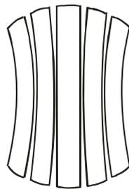
*Fig. 3:* End form of boards after their drying.
