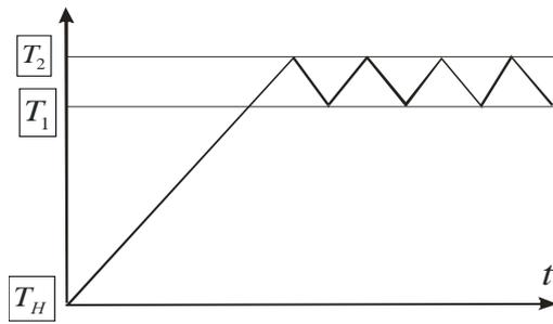
Fig. 15: Temperature graph of cyclic drying regime.
