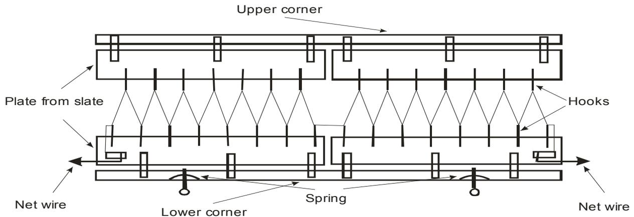
Fig. 12: Construction of electric heater.
