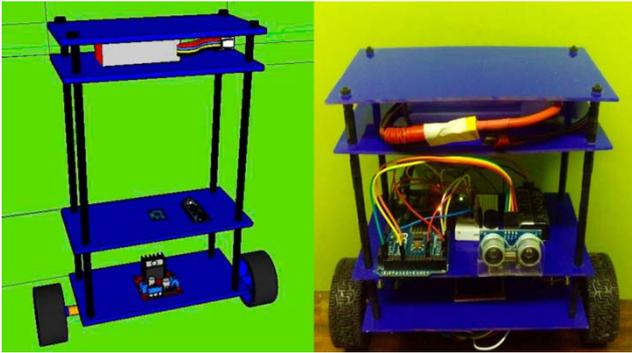
Figure 11: CAD design with the actual hardware implementation
