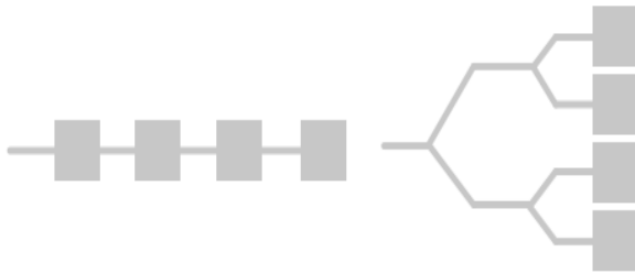
Fig. 1: Series Feed and Corporate Feed Networks.
