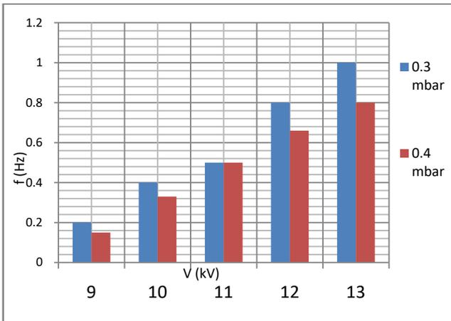
Fig. 12: Variation of repetition frequency for the SORENA-1 PF discharges with discharge voltage. Working gas: D<sub>2</sub>; range of initial pressure: (0.3 - 0.4) mbar.
