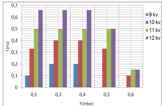
Fig. 10: Variation of repetition frequency for the SORENA-1 PF discharges with initial pressure of working gas. Working gas: Ne; discharge voltage: 9-12 kV.
