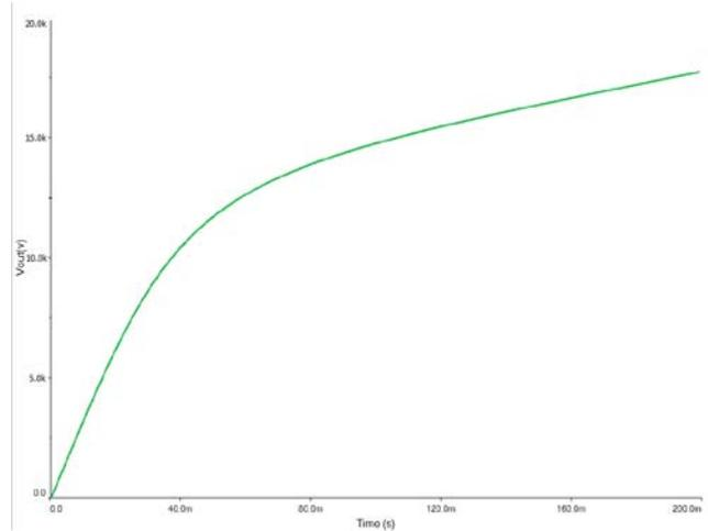
Fig. 14: Charging of capacitor by DC power supply simulated by MultiSim
