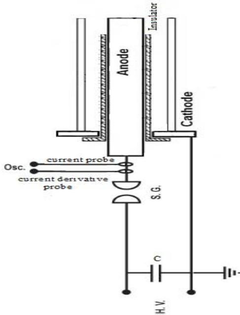
Fig. 1: General structure of electrical connections between capacitor bank and electrodes of SORENA-1.
