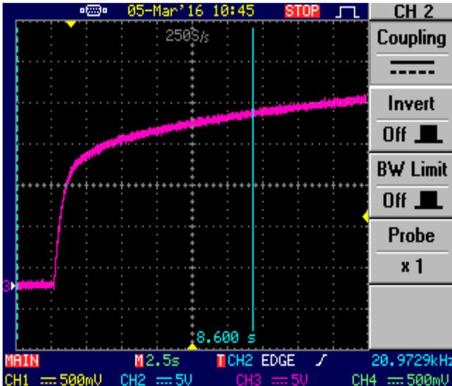
Fig. 13: Charging of capacitor by DC power supply
