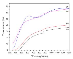
*Fig. 4:* UV-visible transmittance spectrum of  $SnS_2$  thin films deposited at 330 °C using different solutions molar concentration: (a) 0.05 mol/l (b) 0.06 mol/l (b) 0.07 mol/l and (c) 0.08 mol/l.
