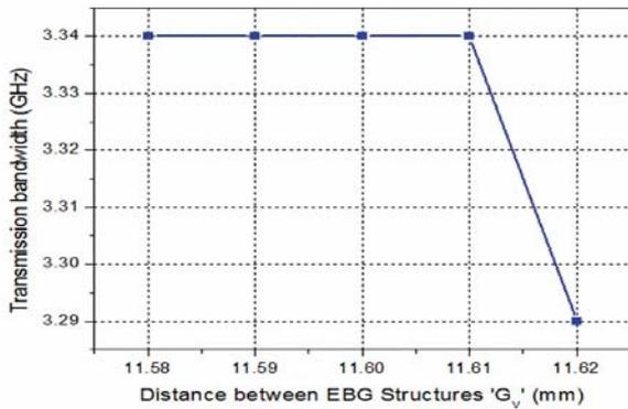
Fig. 16: Distance between EBG structures vs. Transmission Bandwidth of 90° FMSIW filter.
