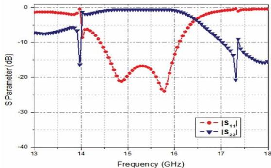
Fig. 10: S-Parameter of 90° FMSIW bandpass Filter with EBG.
