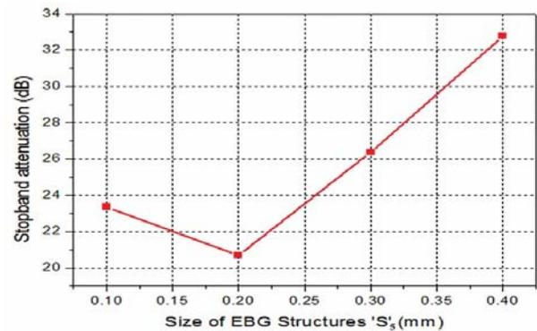
Fig. 19: Size of EBG structures vs. top Band Attenuation of 90° FMSIW Filter.
