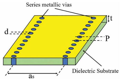
**Fig. 1:** Layout of Basic SIW structure realized on a dielectric substrate ( $a_s$ =effective width of SIW section,  $p$ =center to center gap between vias ‘pitch’,  $d$ =diameter of metallic vias and  $t$ =thickness of dielectric material).
