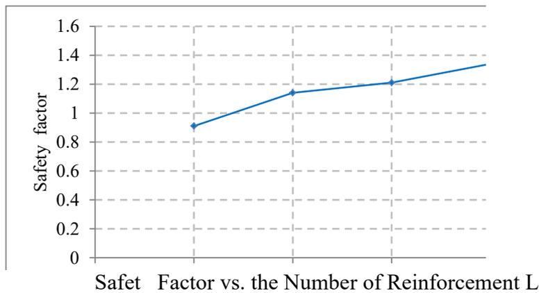
Fig. 4: Changes in Safety Factor vs. the Number of Reinforcement Layers
