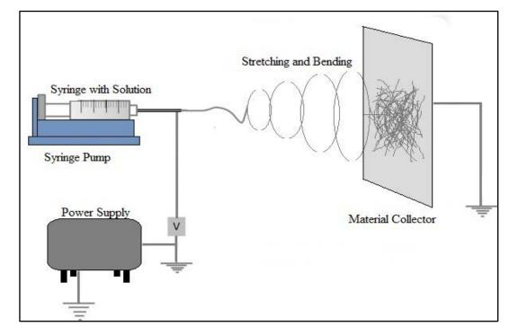
Fig.1: The Electrospinning process schematic
