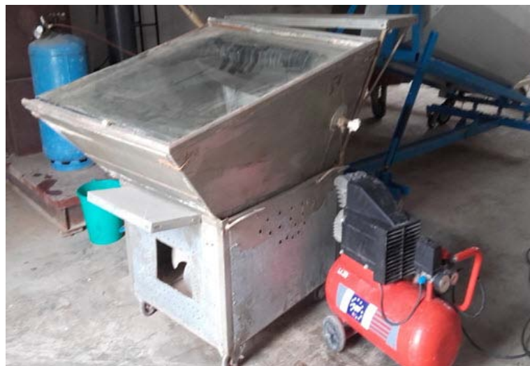
Figure 1b: Actual photograph of SSDHP with air pump
