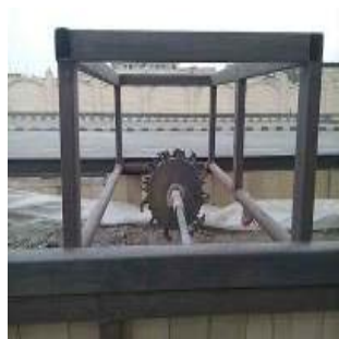
Figure 3: Attaching residue management unit on specified carriage for testing
