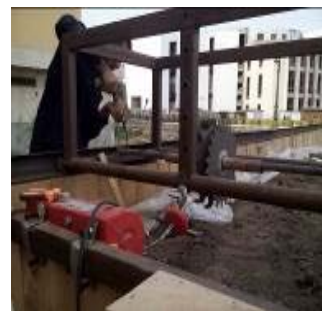
Figure 3: Attaching residue management unit on specified carriage for testing
