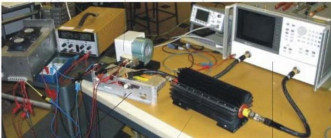
Power amplifier Attenuator Network analyzer
