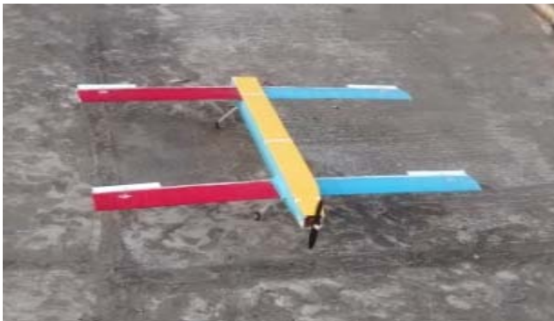
Fig. 21: Prototype made of Composite material and multigrain
