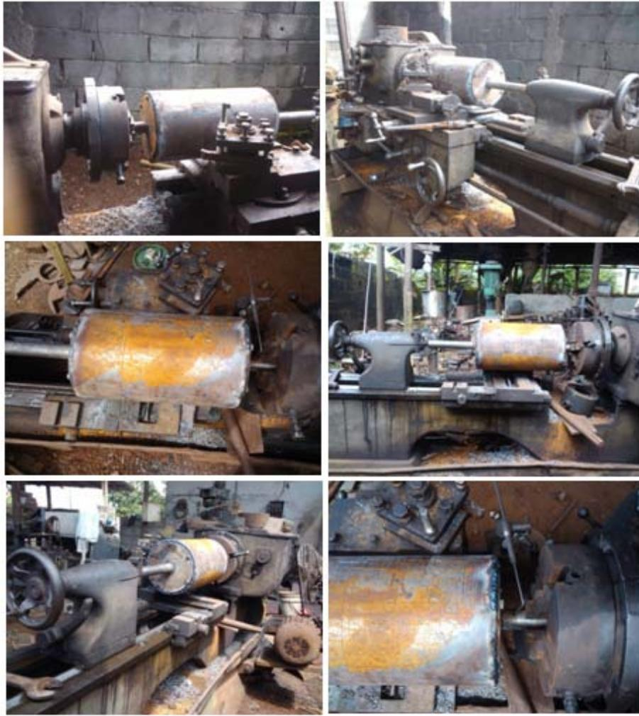
Fig. 9: Different views on how the pipe and flange assembly were mounted on the lathe machine and the scribing of the mounted assembly
