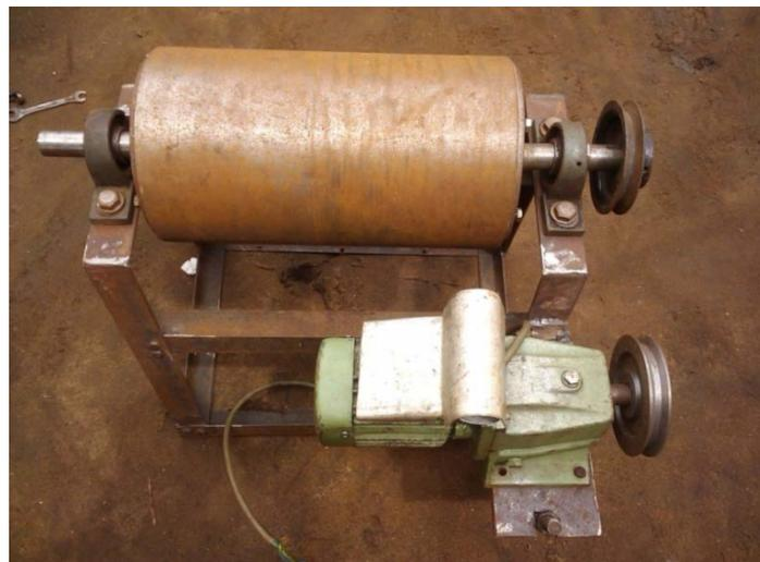
Fig. 15: Complete mill assembly without drive belt
