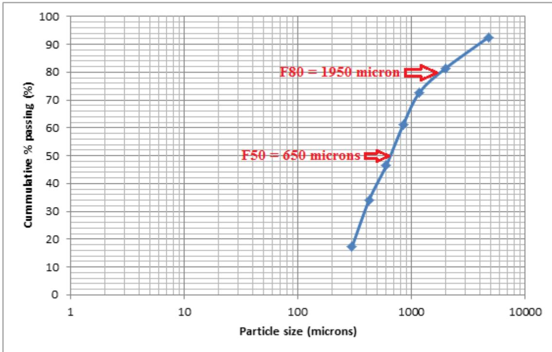
Fig. 18: Graph of Cumulative % passing to Particle size for feed size
