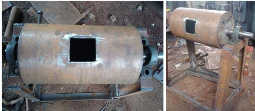
Fig. 12: Feed and discharge hole cut on the vessel
