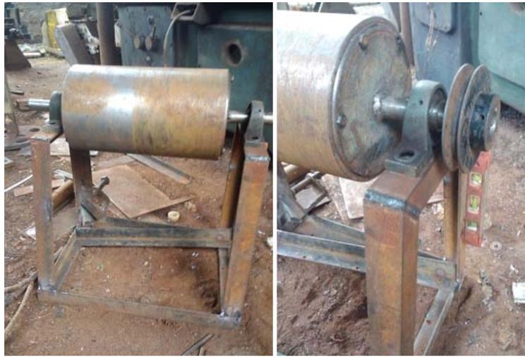
Fig. 11: Mill mounted on the stand
