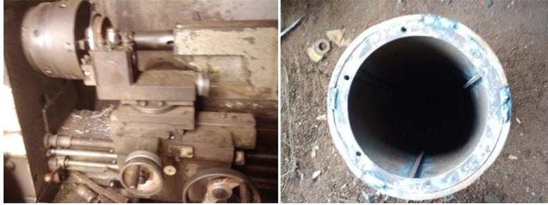
Fig. 5: Marking the rings using the dividing head; machined rings welded to the pipe
