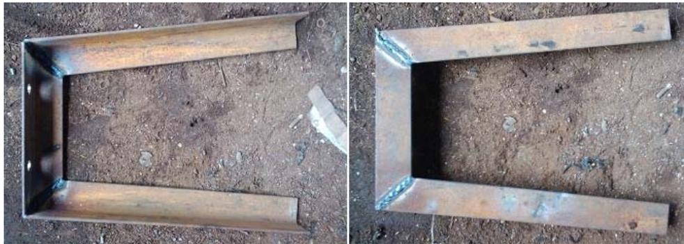
Fig.10: Different views of the welded legs of the stand
