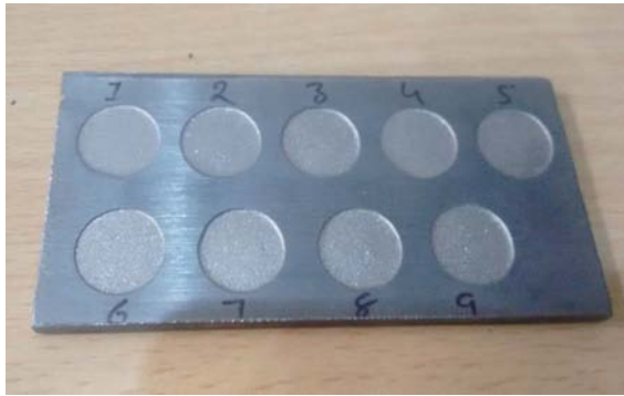
Figure 1: Machined AISI D2 workpiece and aluminium electrode
