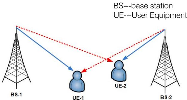
Fig. 2: Joint Transmission CoMP concept.
