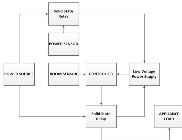
Figure 1: Block Diagram of Automatic Electronic Switching System
