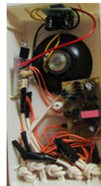
Figure 10: Prototype of the Controller Switch
