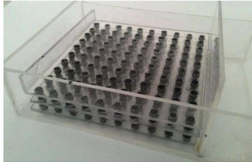
Figure 1: Multi-stack BGA model confined inside a barrier.
