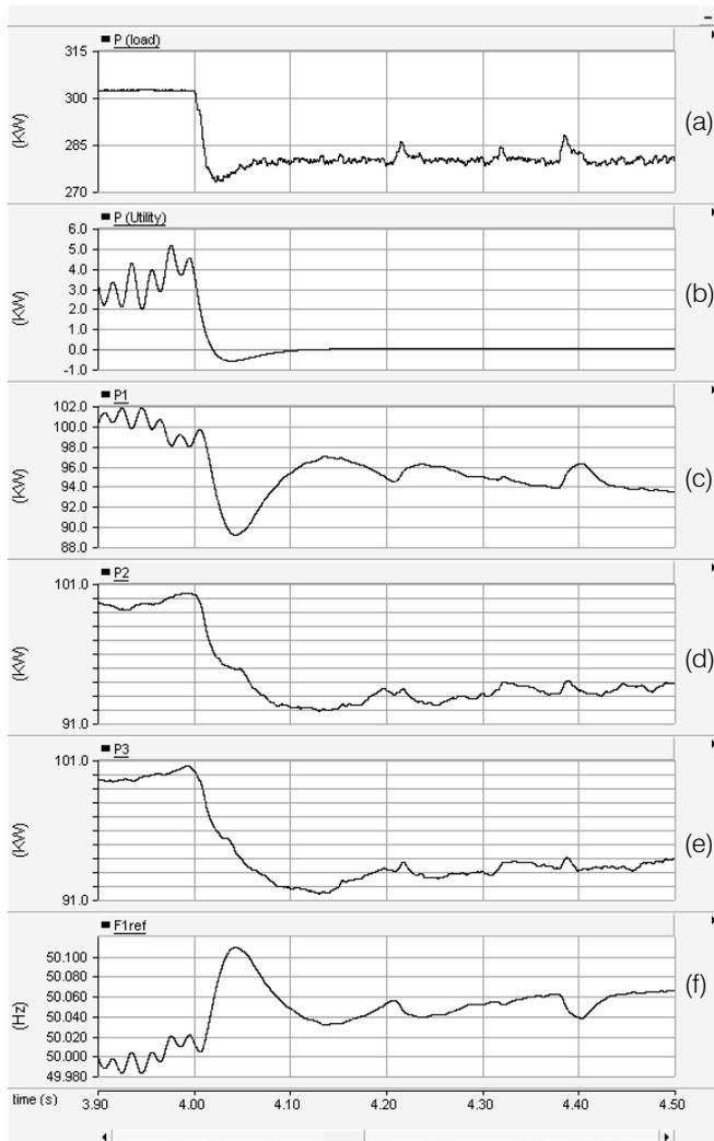
Figure 9: Active power of: (a) load, (b) utility, (c) first DG unit, (d) second DG unit, (e) third DG unit, and (f) frequency of the microgrid during the transition to islanding mode.
