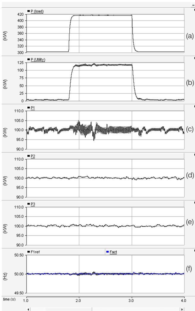
Figure 7: Active power of: (a) load, (b) utility, (c) first DG unit, (d) second DG unit, (e) third DG unit, and (f) frequency of the microgrid during the grid-connected mode.
