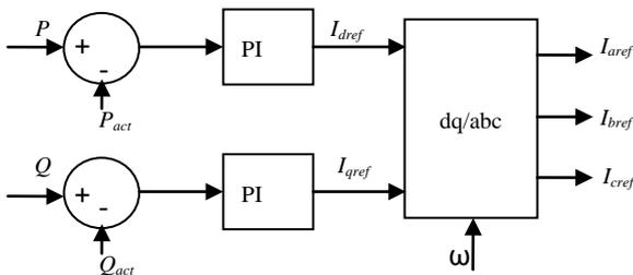
Figure 3: Block diagram of PQ inverter control system
