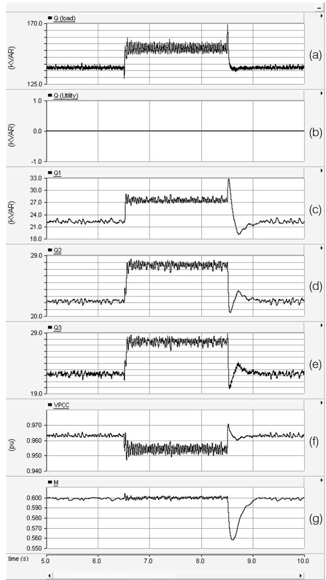
Figure 12: Reactive power of: (a) load, (b) utility, (c) first DG unit, (d) second DG unit, (e) third DG unit, (f) PCC voltage, and (g) modulation index of the first DG inverter during the islanding mode.
