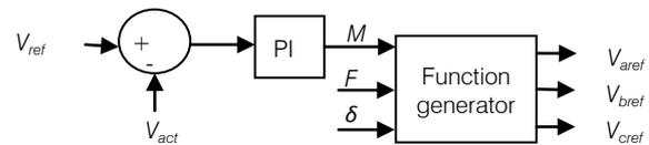
Figure 5: Block diagram of VF inverter control system
