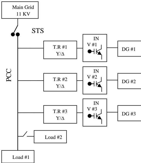
Figure 6: Single line diagram of the proposed system.
