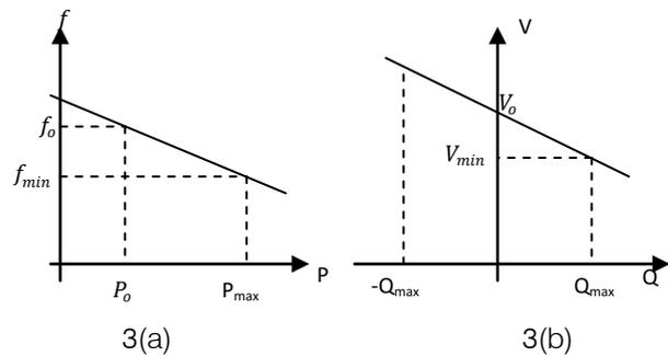
Figure 1: Conventional droop characteristics (a) P-f droop (b) Q-V droop
