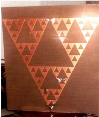
Fig.3.3: Fabricated Sierpinski Monopole Gasket
