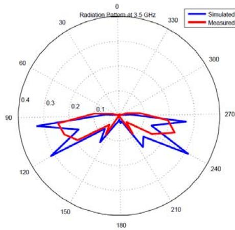
Fig.3.6: Radiation Pattern at 3.5 GHz
