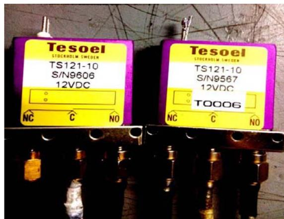
Fig 4.7: Teseol SPDT switches
