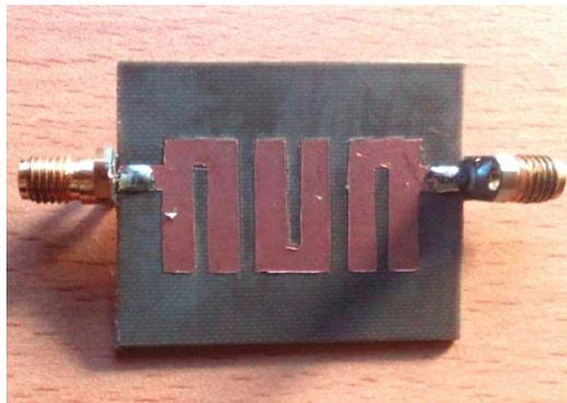
Fig 4.2: Fabricated 3.5 GHz Filter
