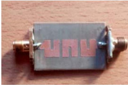
Fig 4.4: Fabricated 7.5 GHz Filter
