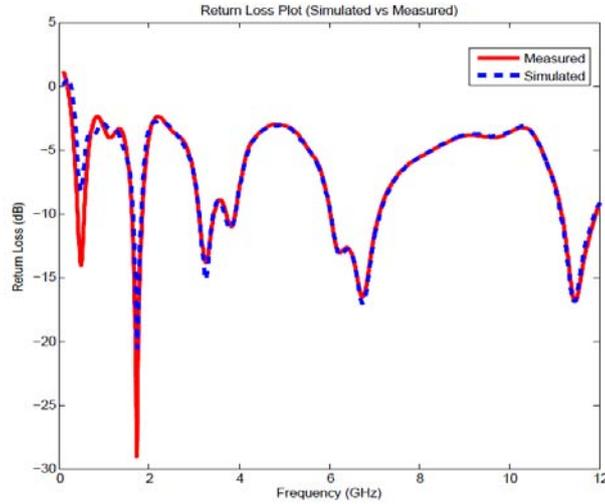
Fig.3.4: Simulated and Measured Return Loss Plot
