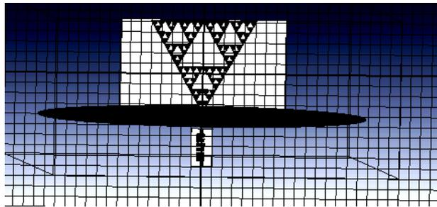
Fig 5.2: Antenna with 7.5 GHz Filter Simulation
