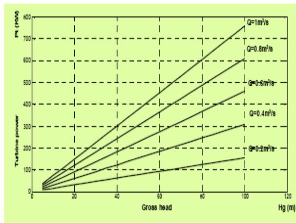
Figure 11: Variation of turbine power with gross head at different values of water flow rate
