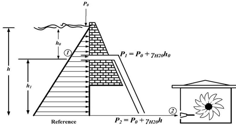
Figure 9: Variable Pressure by Water Height
