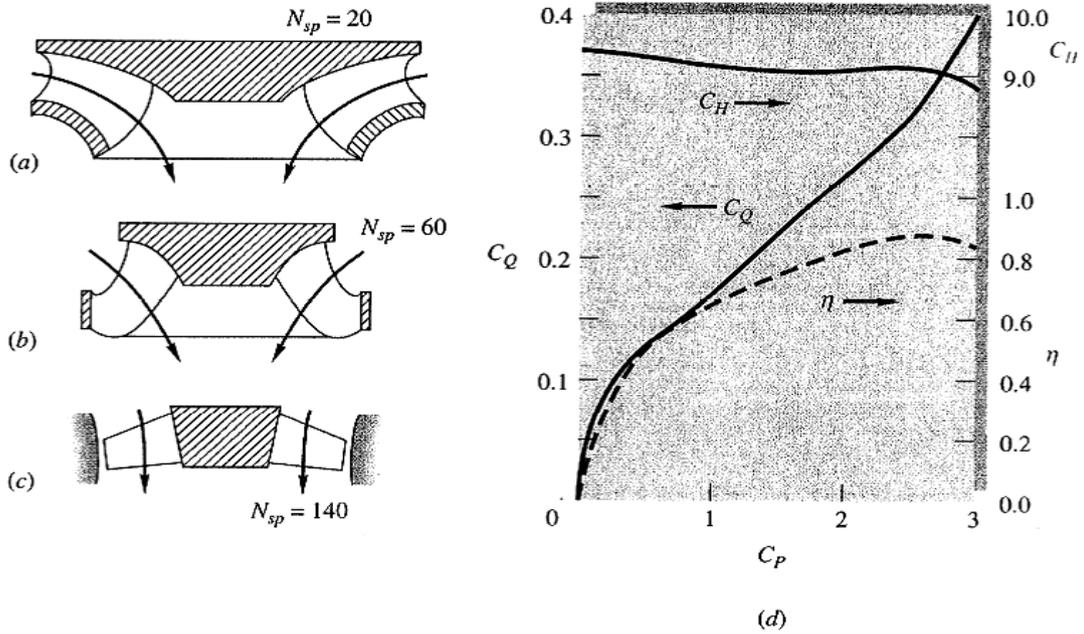
Fig. 4: Reaction turbines: (a) Francis, radial type; (b) Francis, mixed-flow; (c) propeller axial-flow; (d) performance curves for a Francis turbine,  $n = 600$  rpm,  $D = 0.686$  m,  $N_{sp} = 29$ .
