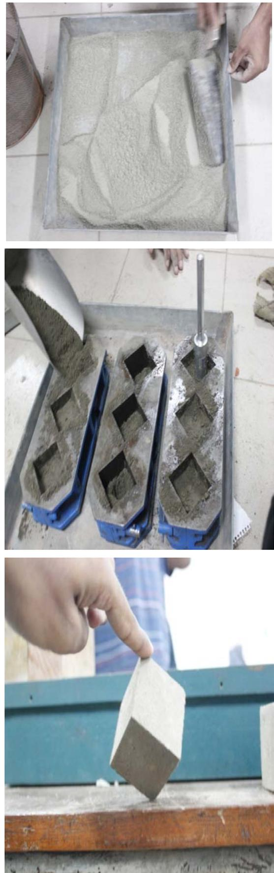
Fig. 2: Final Sample of Soil-Cement Block
