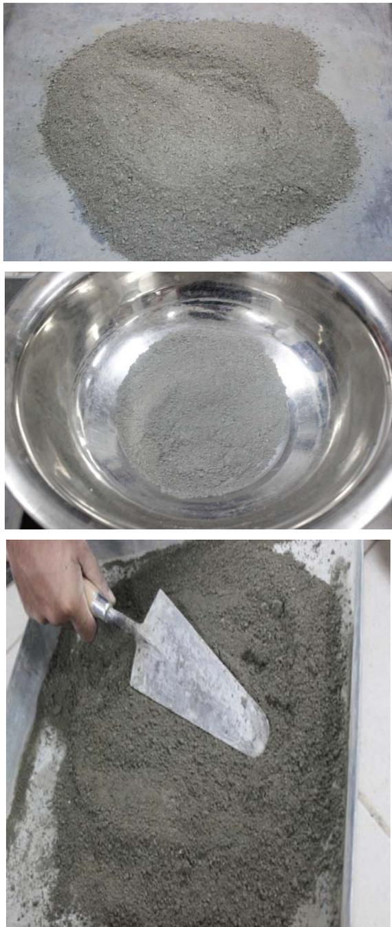
Fig. 1: Soil Cement Mixing and Moulding
