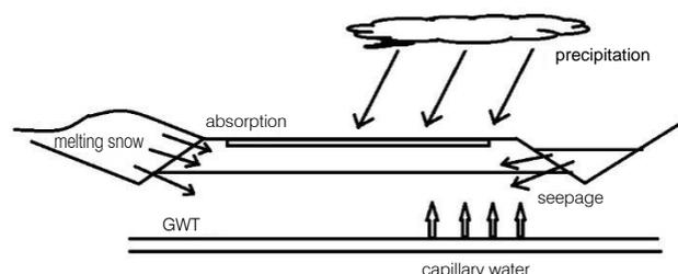
Fig. 1: Main Sources of Water in Pavement
