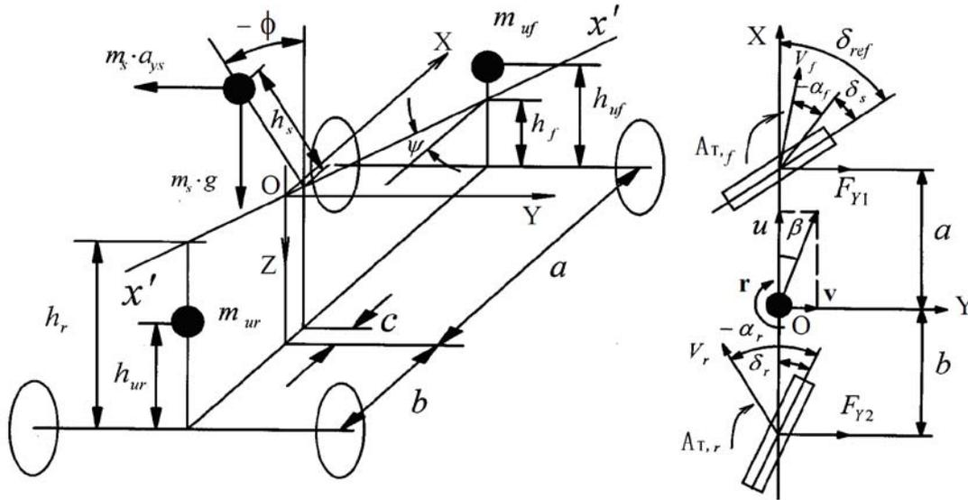
Fig. 2: Linear 3-dof vehicle handling model
