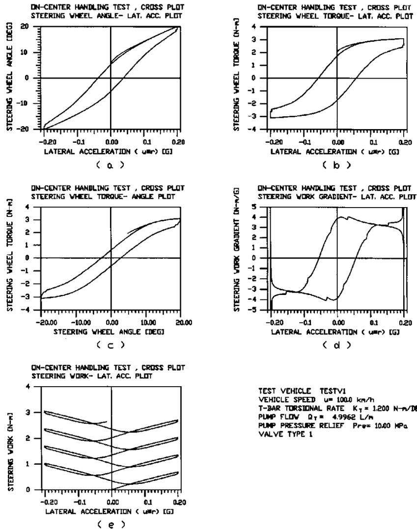
Fig. 11: On-center handling cross-plots ( $Q_T = 4.996$  L/m)
