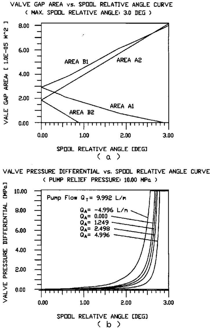
Fig. 6: Valve areas and pressure differential characteristics
