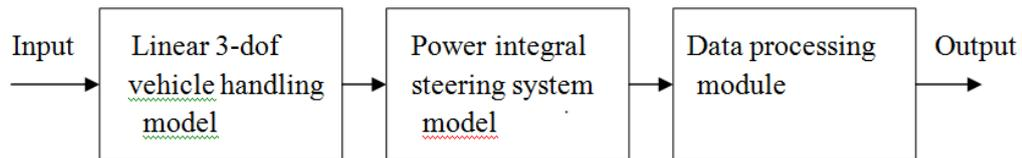
*Input:* reference steer angle of vehicle front wheels
