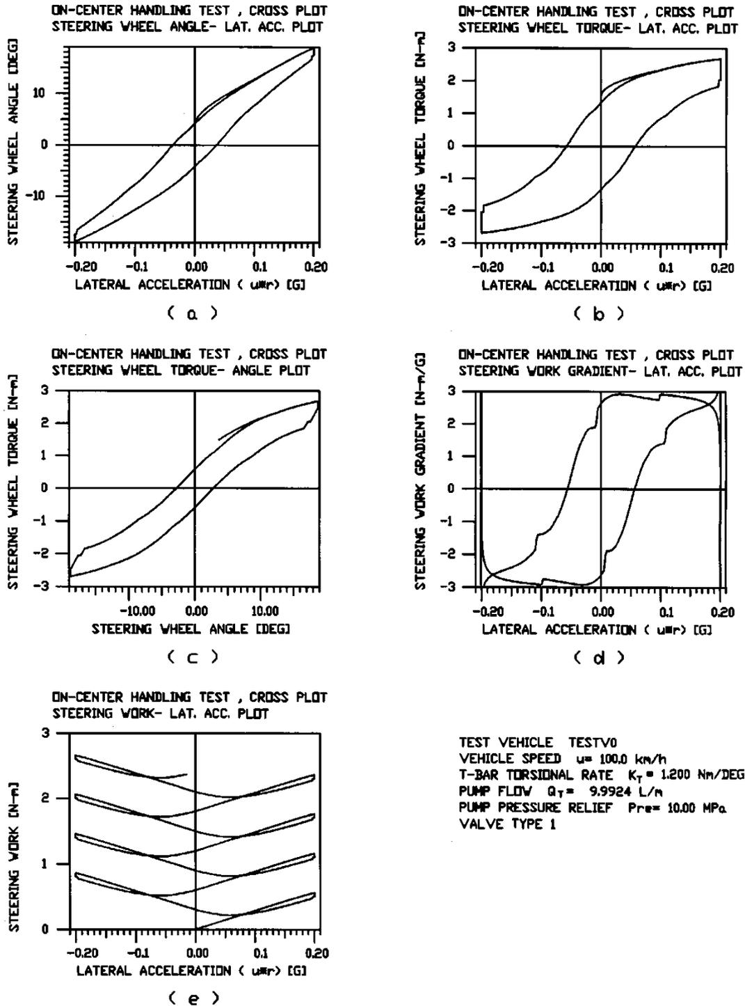
Fig. 10: On-center handling cross-plots ( $Q_T=9.992$  L/m)
