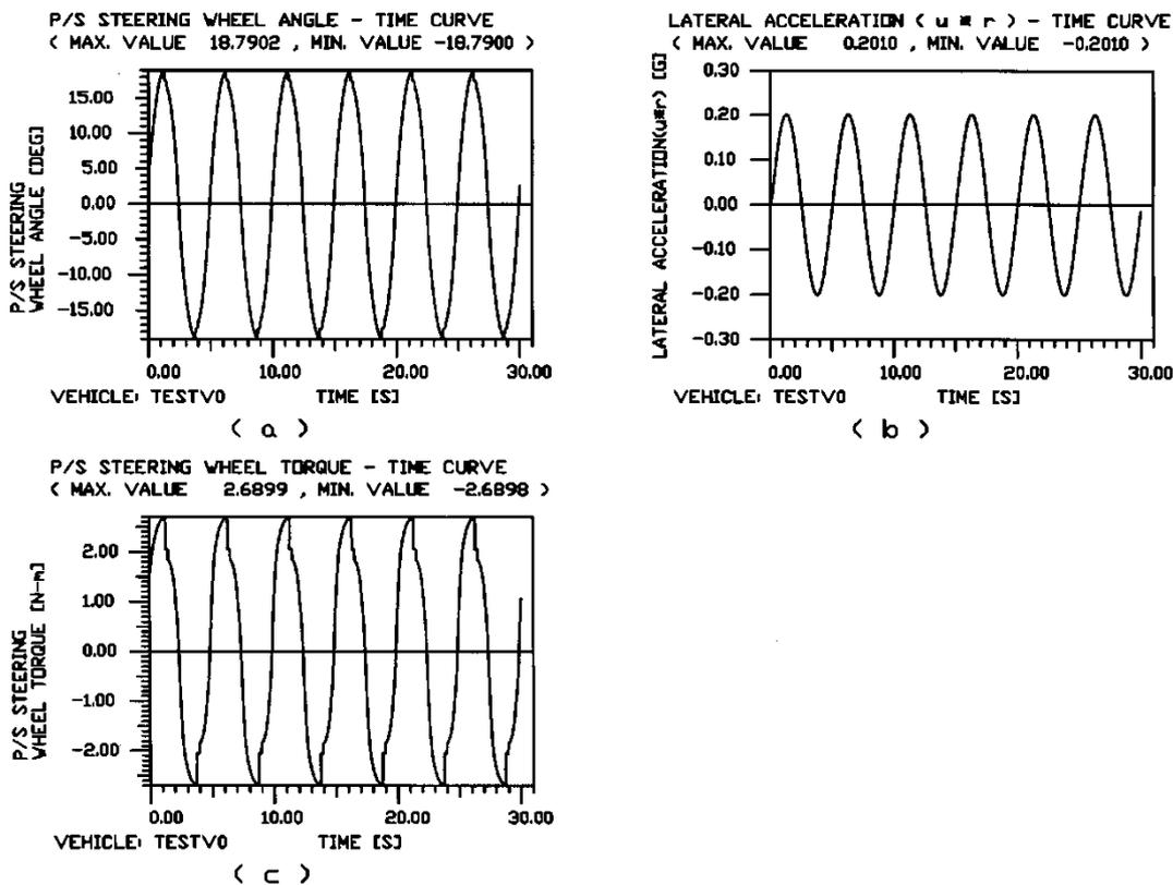
Fig. 9: Time histories of  $\delta_{SW}$ ,  $T_{SW}$ , and lateral acceleration  $a_y(u \cdot r)$
