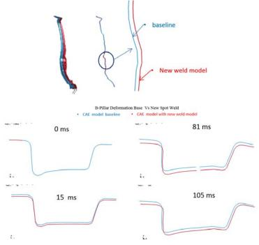
Fig.8: Post-crash deformation of the B-Pillar spot weld welded structures
