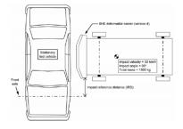
Fig.6: Moving deformable barrier alignment with test vehicle [26]
