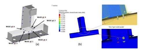
Fig. 5: (a) Location of spot weld on specimen, (b) weld failure captured from the simulation
