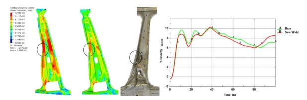
*Fig.* 9: (a)Comparison of Stress contour of the B-Pillar spot weld welded structures LH side view, (b) Test Deformation of the B-Pillar[27] RH side view, (c)B-pillar velocity comparison
