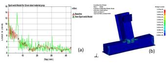
Fig. 3:(a) Force response of simulation loading (Baseline and New spot weld), (b) New spot weld post deformation
