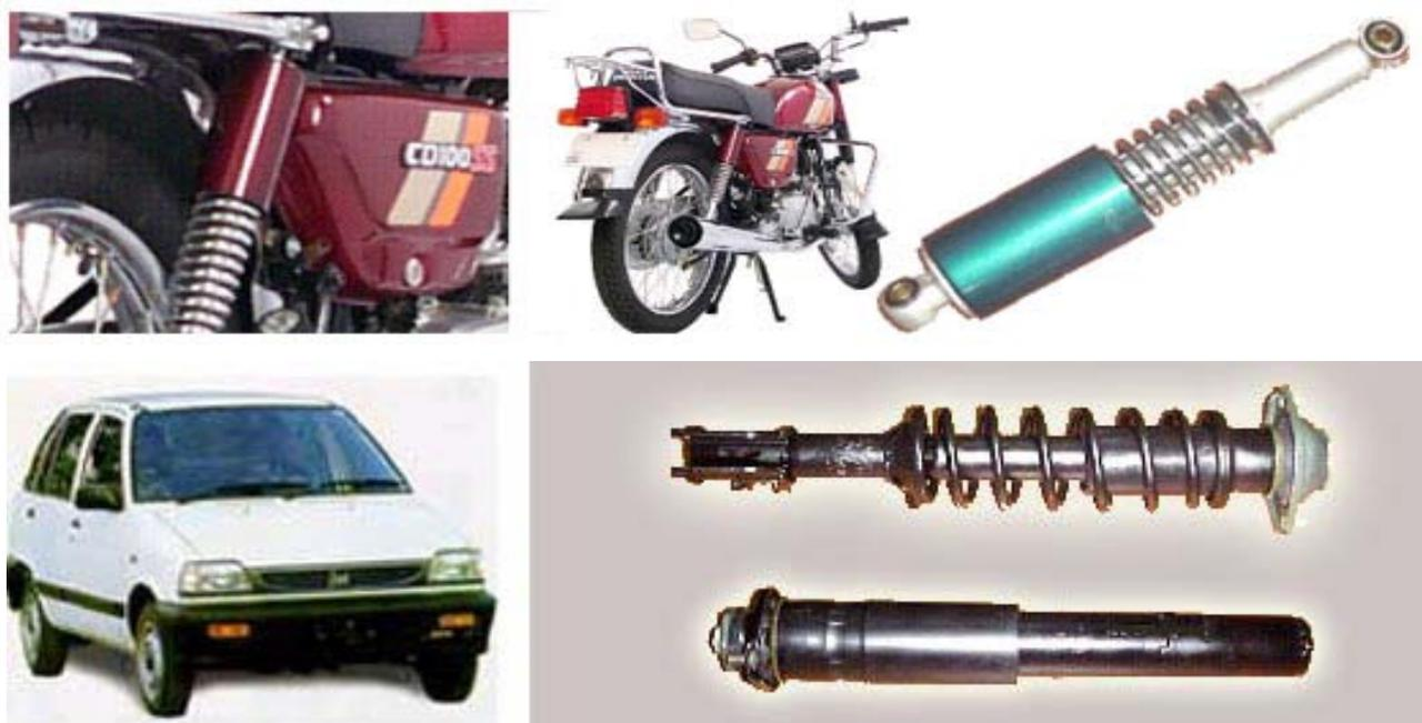
Figure 2 : Photographs of two and four wheeler shocker
