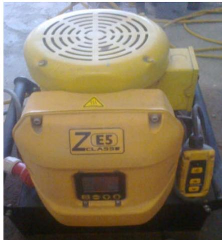
Figure 2 : The loading device (model Enerpac-ZE5)
