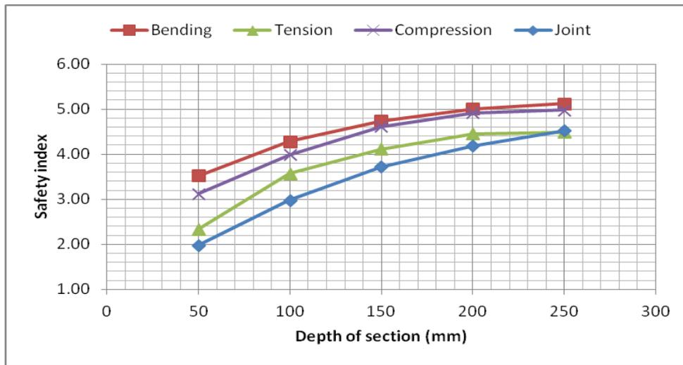
Figure 2 : Variation of safety index against depth of section for *Mansonia altissima*
