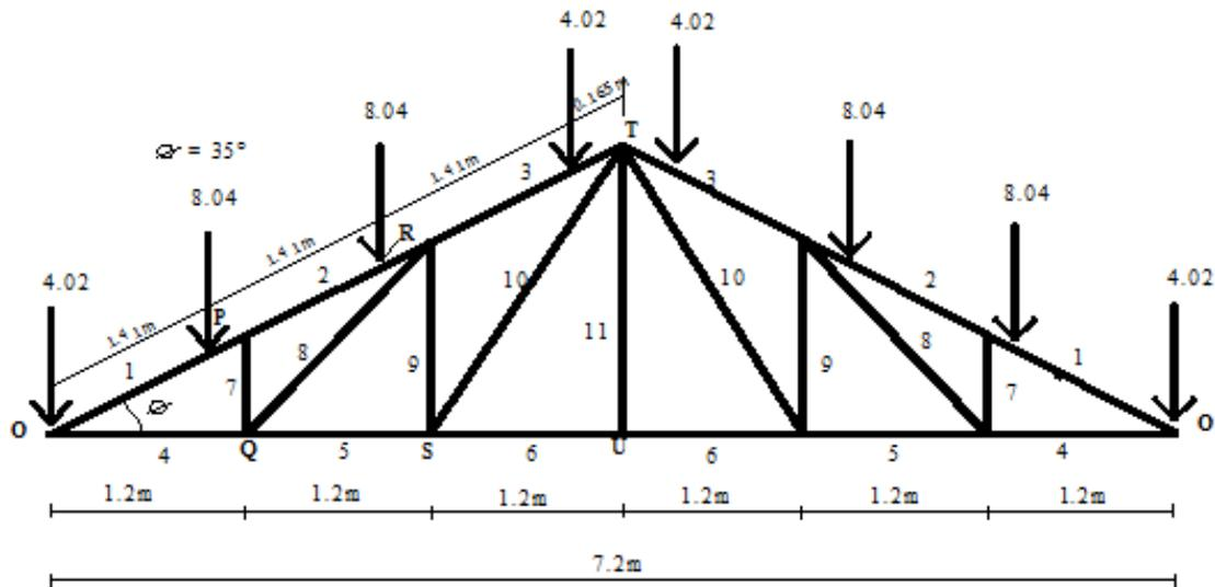
Fig. 1 : Typical truss subjected to nodal design loadings
