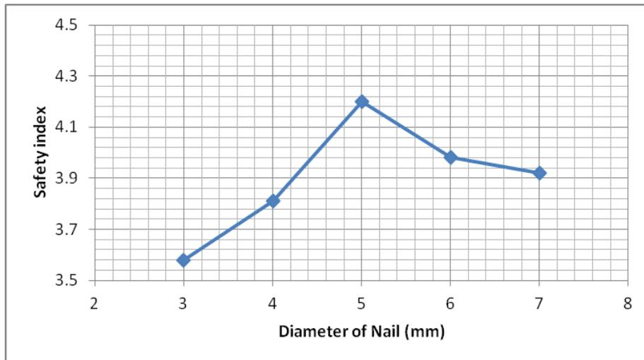
Figure 5 : Variation of safety index with diameter of nail
