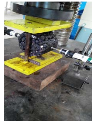
Figure 6 : Test Indirect Tensile Strength
