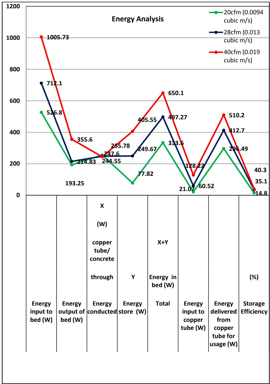
Figure 7.0 : Energy analysis of simultaneous charging and discharging packed bed storage system at airflow rate of 0.0094, 0.013, and 0.019m<sup>3</sup>/s for 0.065m diameter spherical shaped concrete
