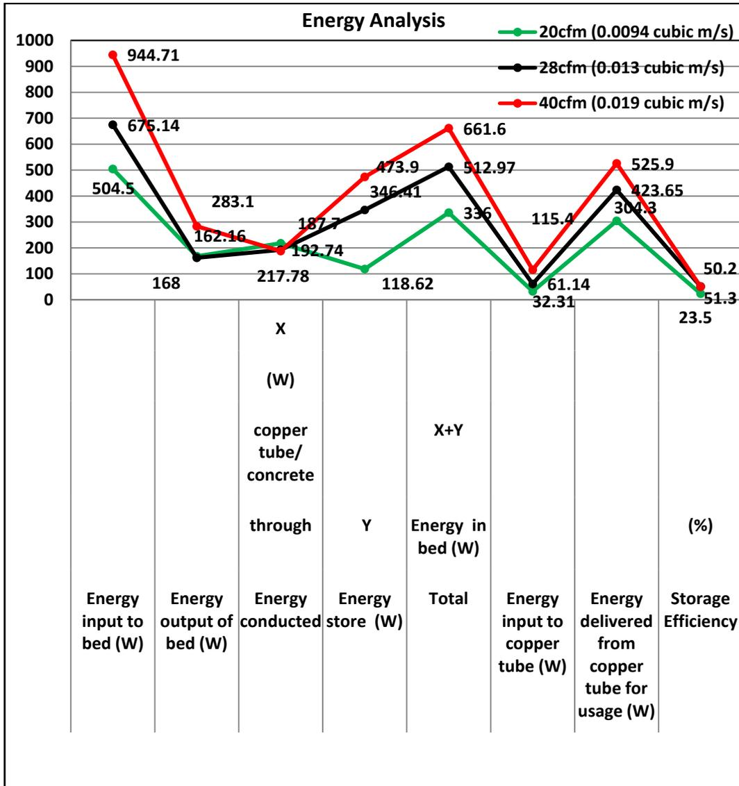
Figure 6.0 : Energy analysis of simultaneous charging and discharging packed bed storage system at airflow rate of 0.0094, 0.013, and 0.019m<sup>3</sup>/s for 0.08m diameter spherical shaped concrete
