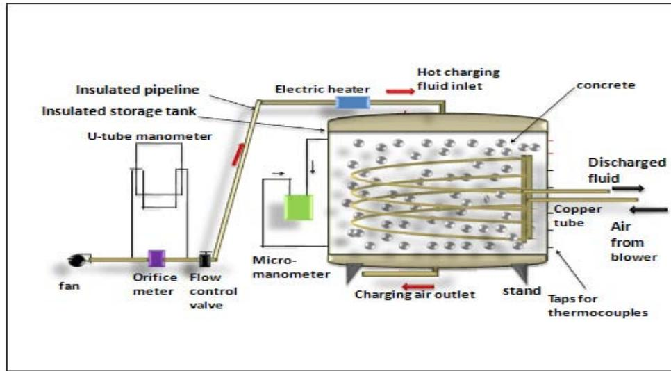
Figure 2.0: A diagrammatic sketch of simultaneous charging and discharging packed bed energy storage system components
