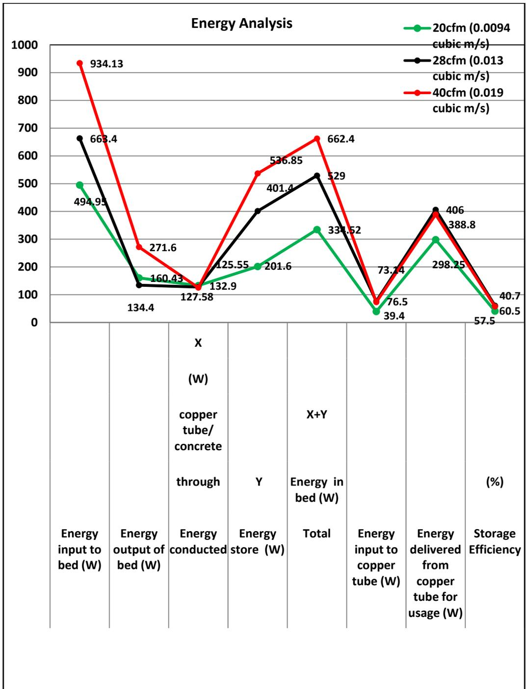
Figure 5.0 : Energy analysis of simultaneous charging and discharging packed bed storage system at airflow rate of 0.0094, 0.013, and 0.019m³/s for 0.11m diameter spherical shaped concrete
