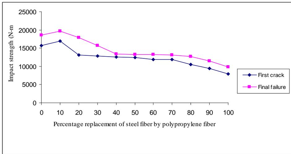
Figure 3 : Variation of impact strength of slurry infiltrated fibrous ferrocement with partial replacement of steel fiber by polypropylene fiber.
